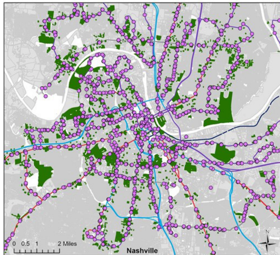
Figure 1. Final output layer of identified potential land area within a 0.25-mile buffer of Nashville’s public transportation network.
